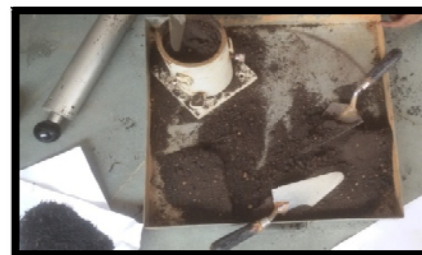
Fig. 11 Compaction Test Equipments
